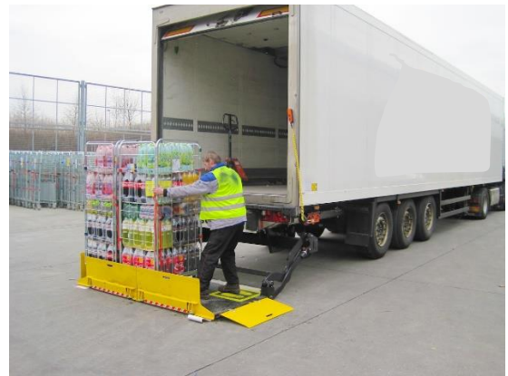
Example of a delivery vehicle tail lift © Dhollandia
