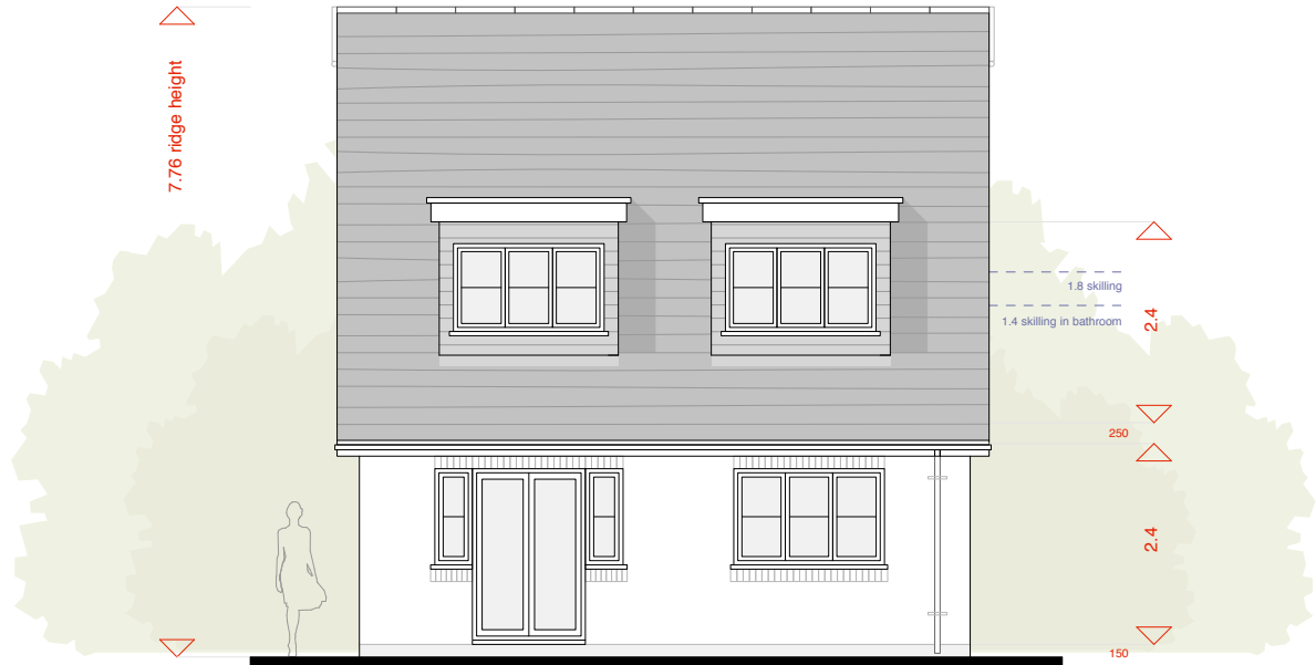
Proposed Rear Elevation at 1:100 scale EAST
