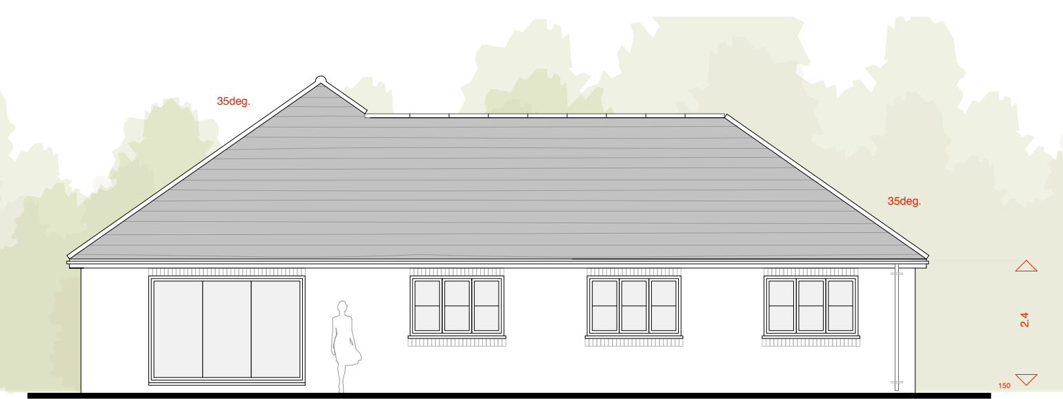
Proposed Rear Elevation at 1:100 scale WEST
