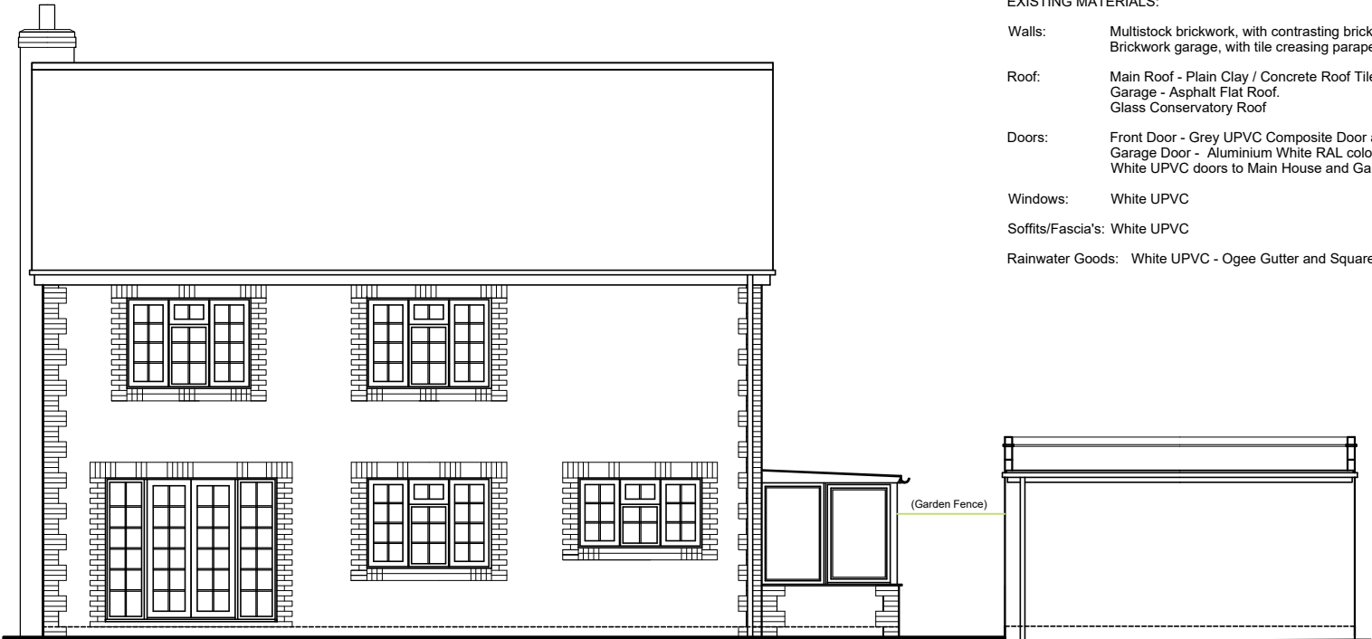
Existing South East Elevation
