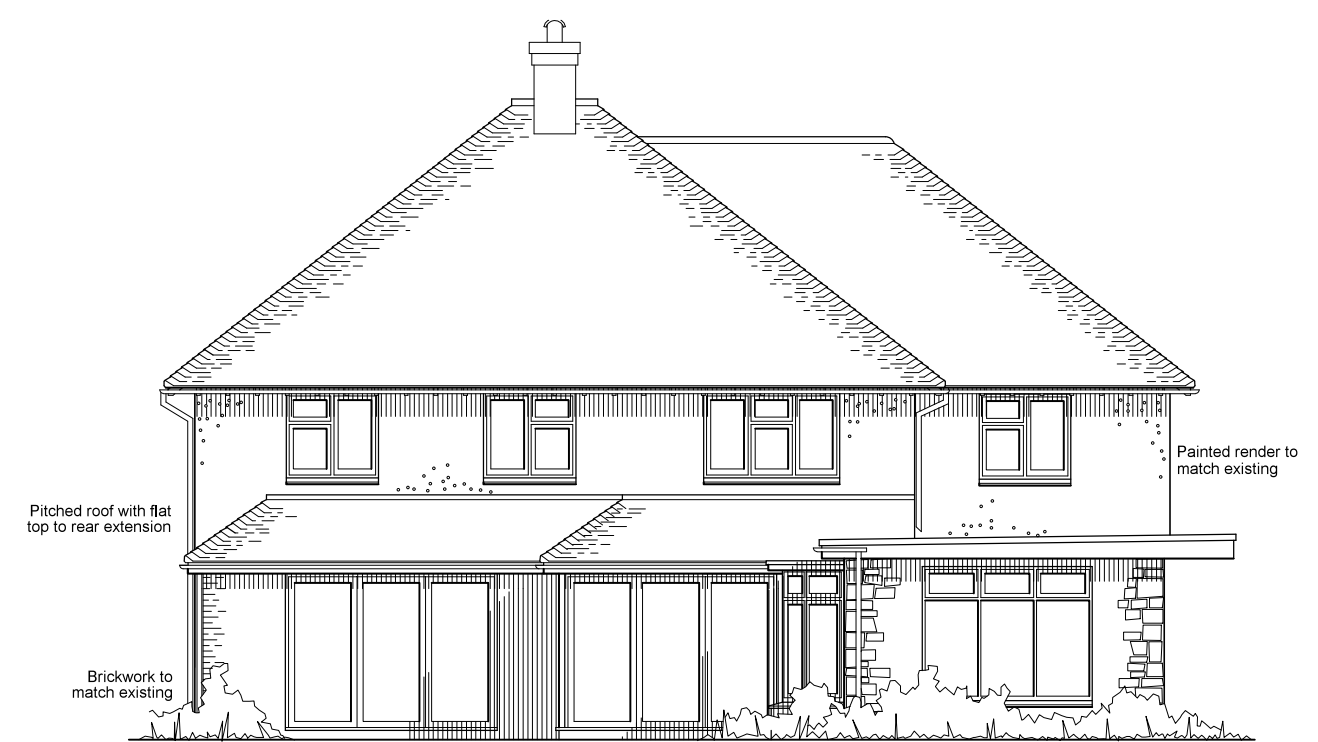
North West Elevation
