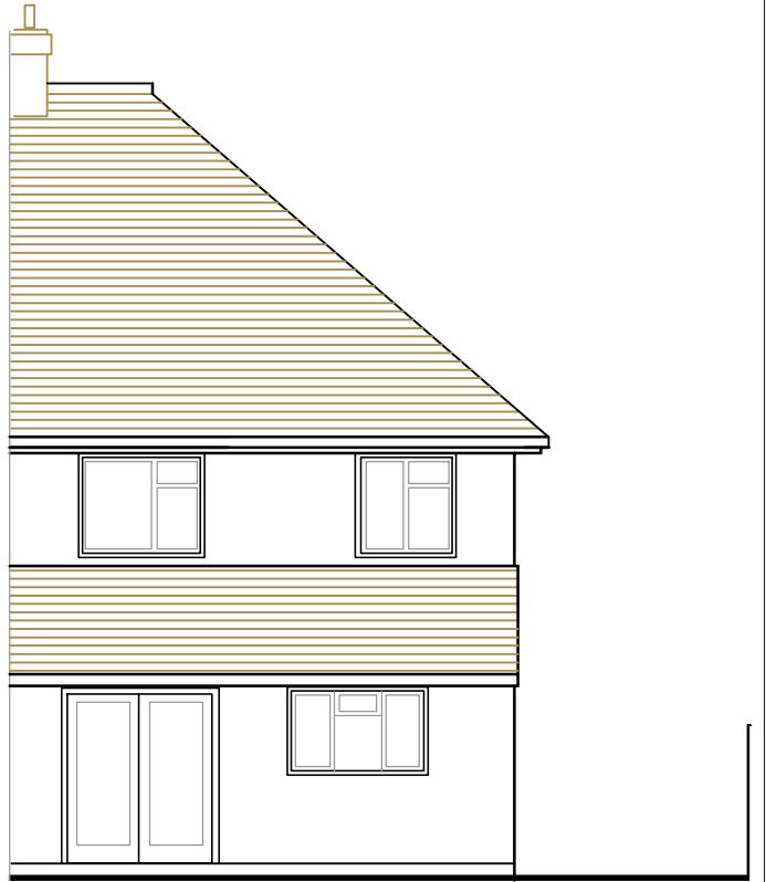
EXISTING SOUTH ELEVATION 1:100
