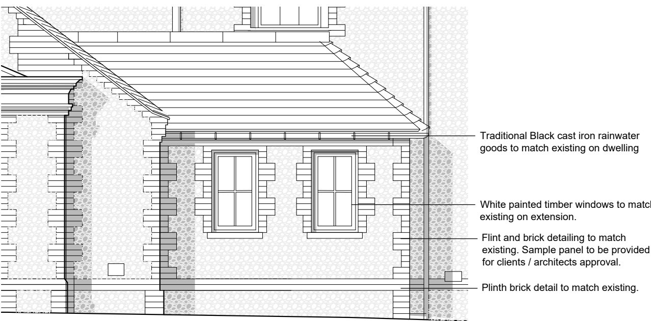
BOOT ROOM DETAIL NORTHEAST ELEVATION scale 1_50
