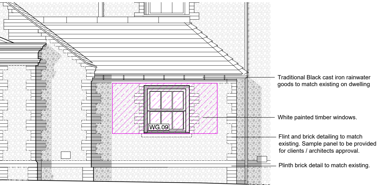
BOOT ROOM DETAIL NORTHEAST ELEVATION scale 1_50
