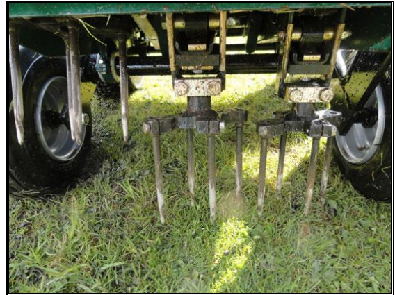
Plate 8: Pedestrian aerator fitted with solid tines
