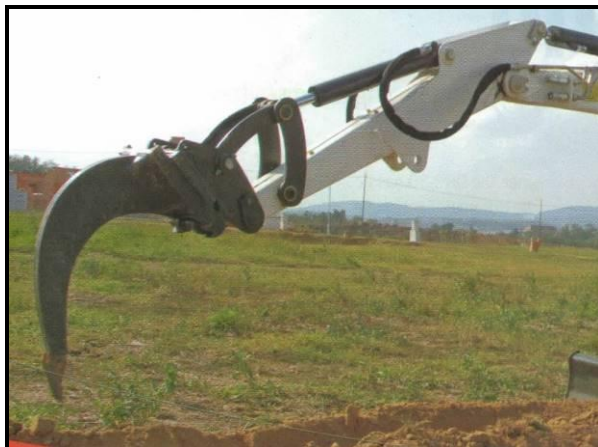
Plate 1: Excavator arm fitted with a Single Tine Ripper Attachment
