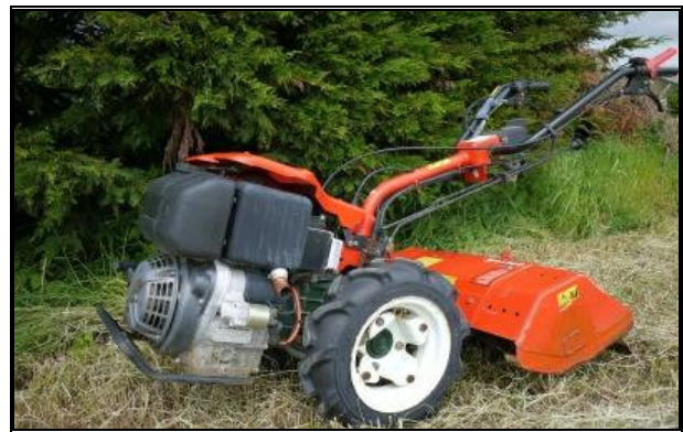
Plate 6: Example of pedestrian rotovator
