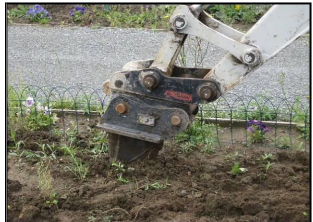
Plate 2: Single Tine Ripper working
