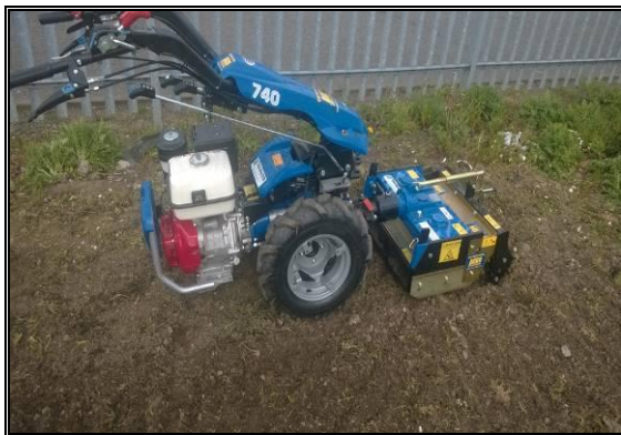
Plate 5: Example of power harrow
