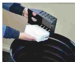
Remove and replace spent Smart Pak
