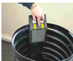
Install new Smart Pak and refit
