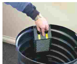
Remove the front plate by sliding upward
