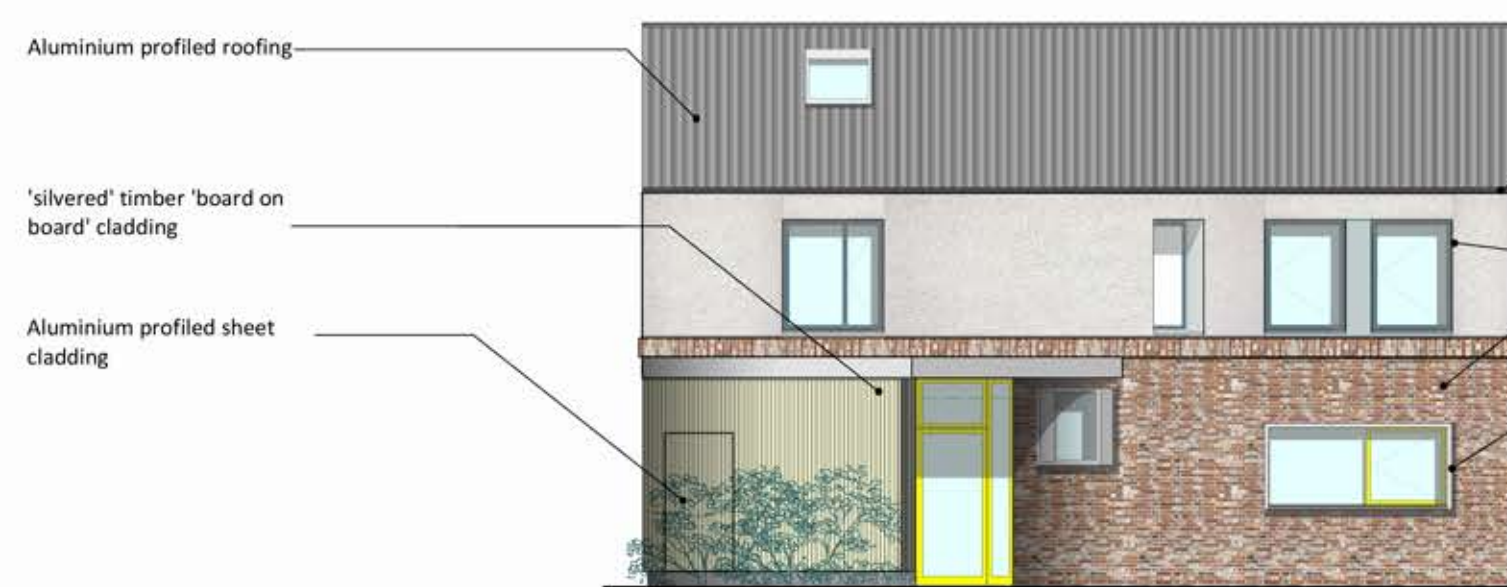
North/North East Elevation
