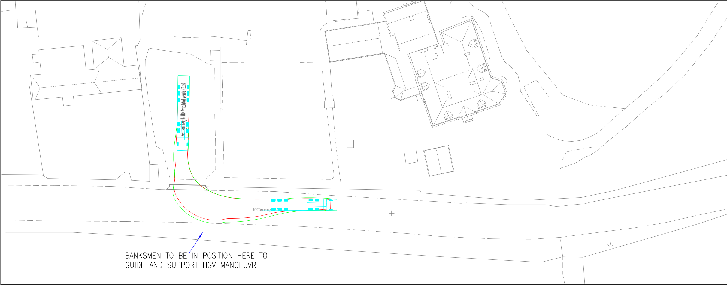
16.5M ARTICULATED VEHICLE EXITING THE SITE
