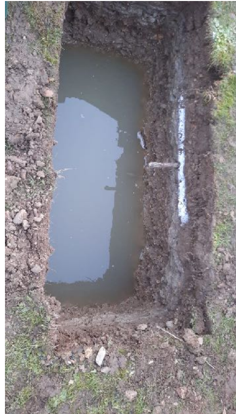
Pit showing 25% and 75% levels for measuring water absorption and image of the pit during the test
