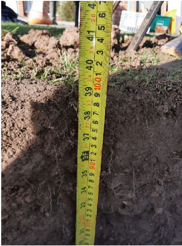
Evidence of test pit depth and pit showing strata
