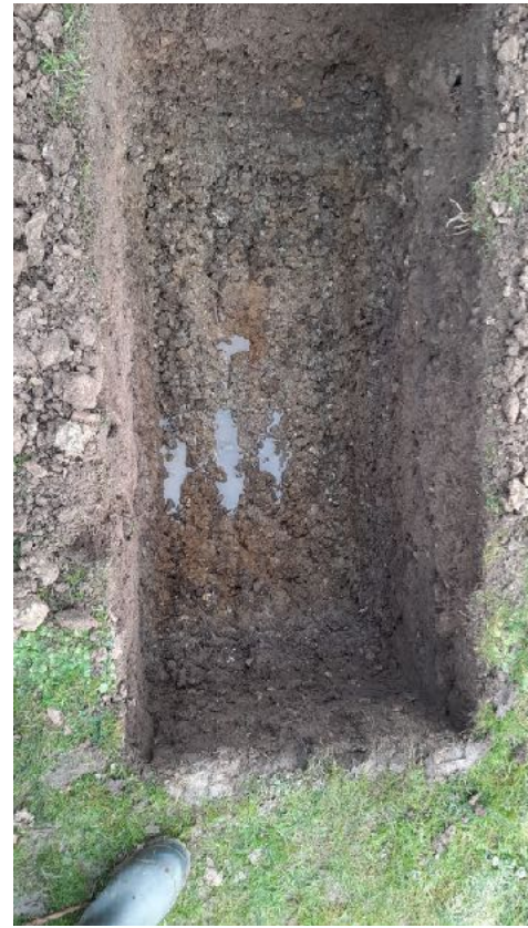
Evidence of test pit depth and pit showing strata
