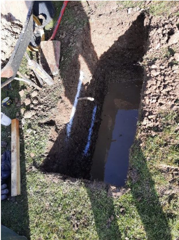
Pit showing 25% and 75% levels for measuring water absorption and image of the pit during the test
