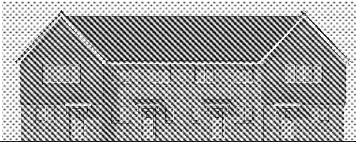
Short Terrace, mixture of brick and tile hanging
