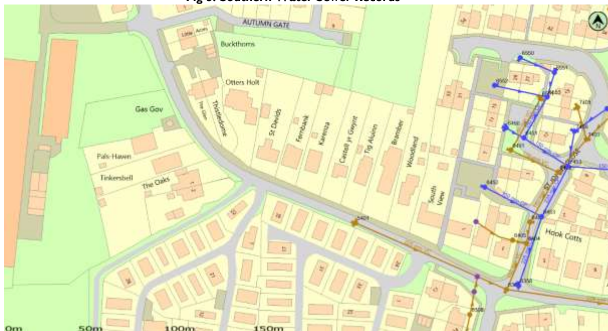
Fig 3. Southern Water Sewer Records
