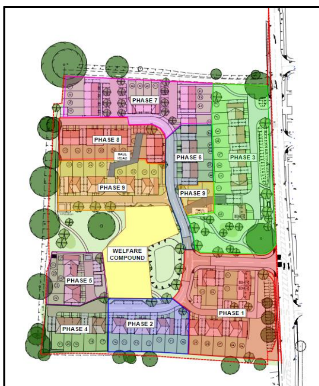
Figure 2: Construction Phase Plan
