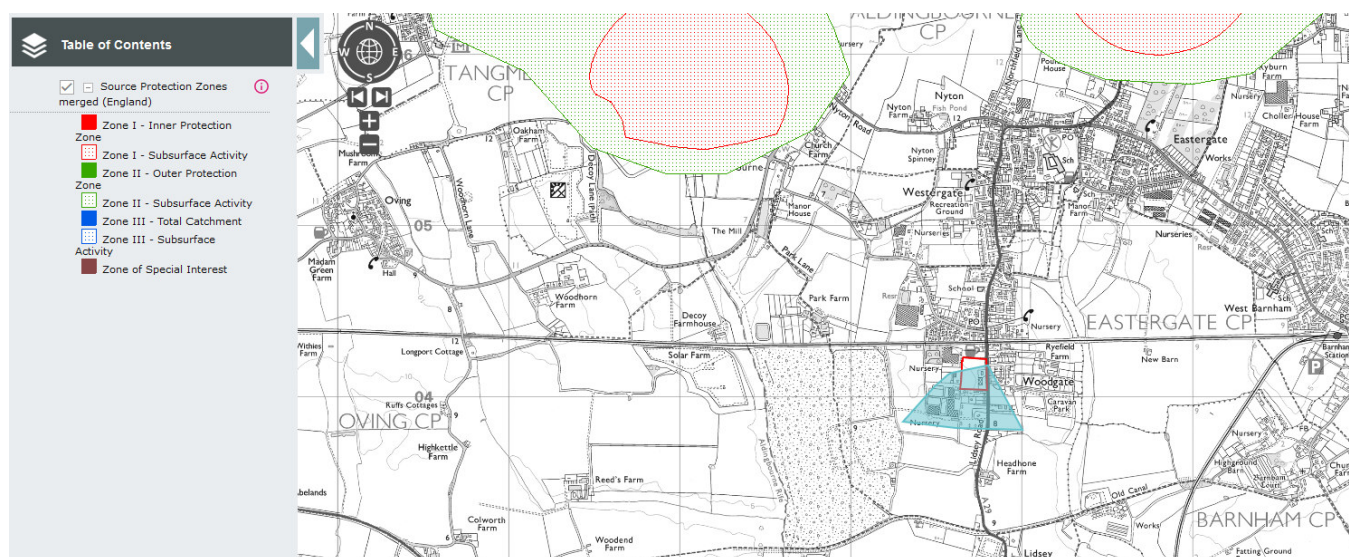
Figure 7. DEFRA Groundwater Source Protection Zone Map
