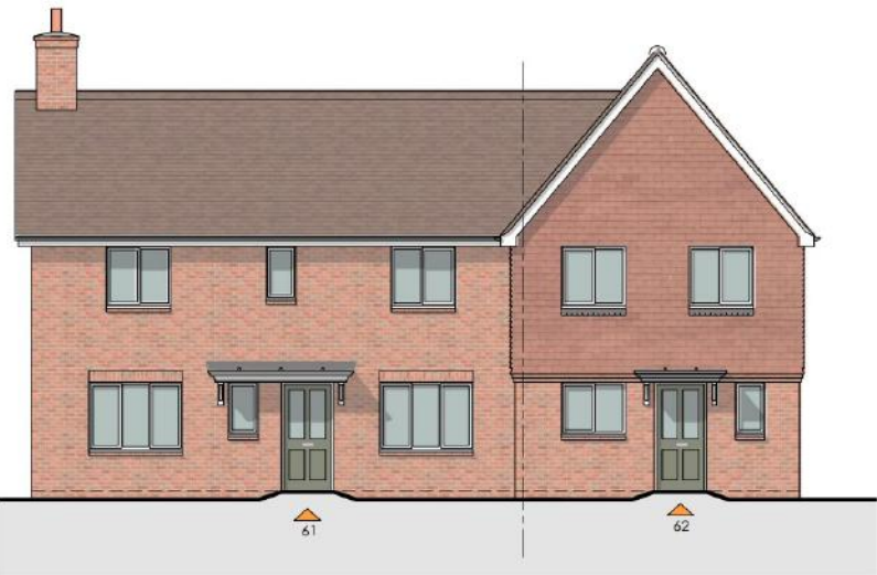
Semi-detached mixture of brick and tile hanging
