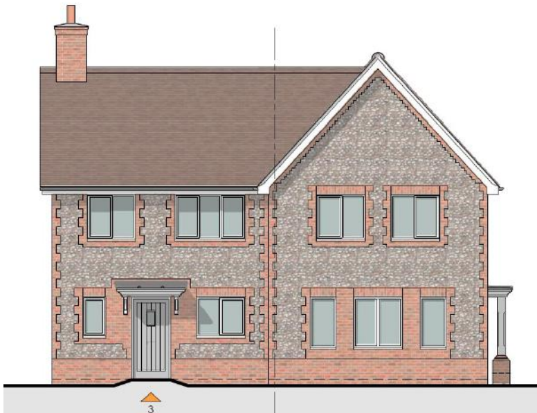
Semi-detached, flint feature detailing
