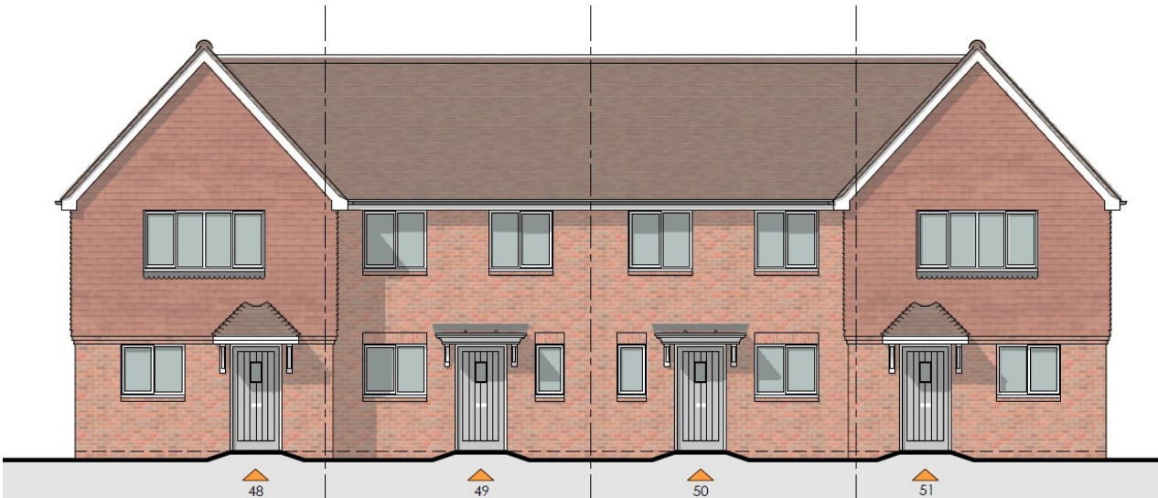
Short Terrace, mixture of brick and tile hanging
