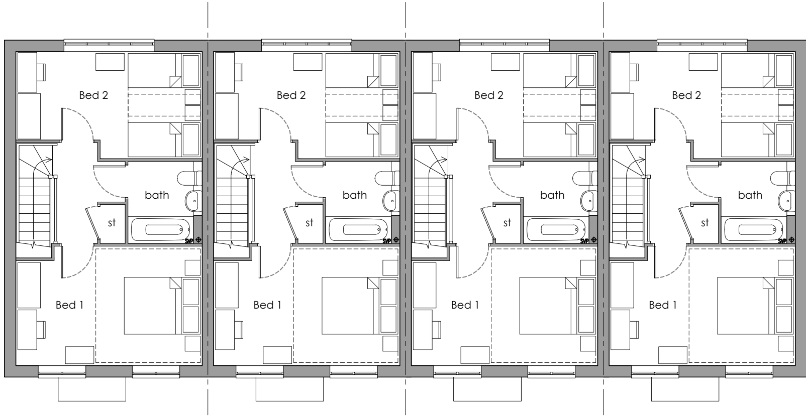
FIRST floor plan
