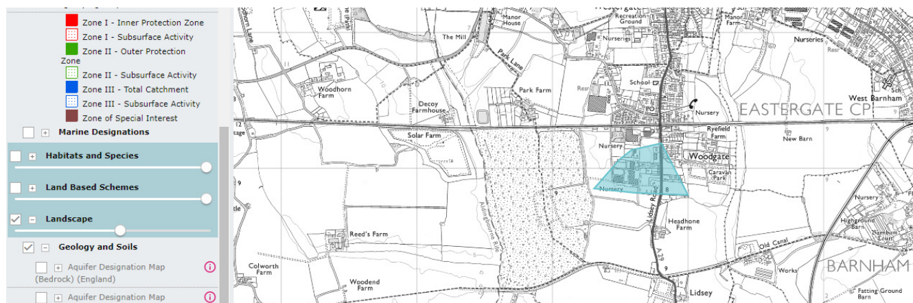
Figure 7. DEFRA Groundwater Source Protection Zone Map
