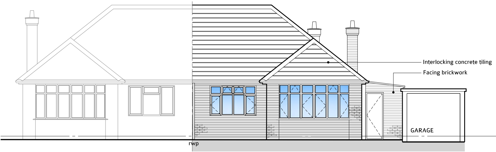
FRONT (north) ELEVATION AS EXISTING 1:100
