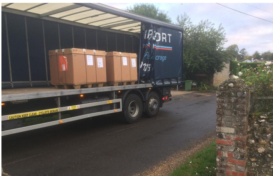
Photograph showing delivery vehicle obscuring the sight line of vehicles leaving Old Dairy Lane (the wheely bin is at the entrance to Old Dairy Lane).
