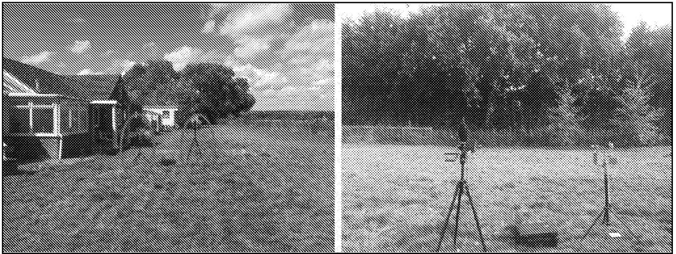
Figure 4. Monitoring location with direct line of sight of the railway lines with the microphone and weather station shown
