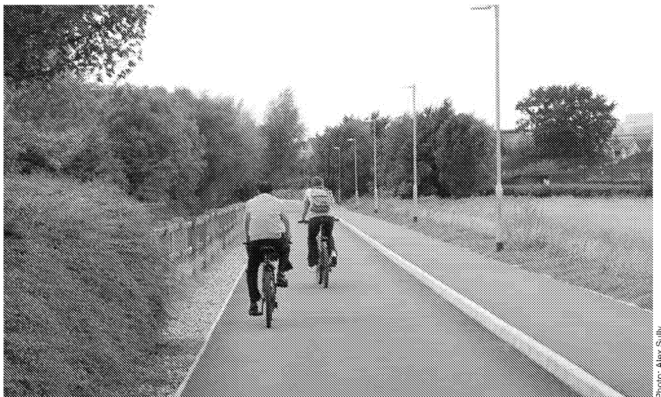
Figure 7.3 Shared use segregated by kerbed level difference
