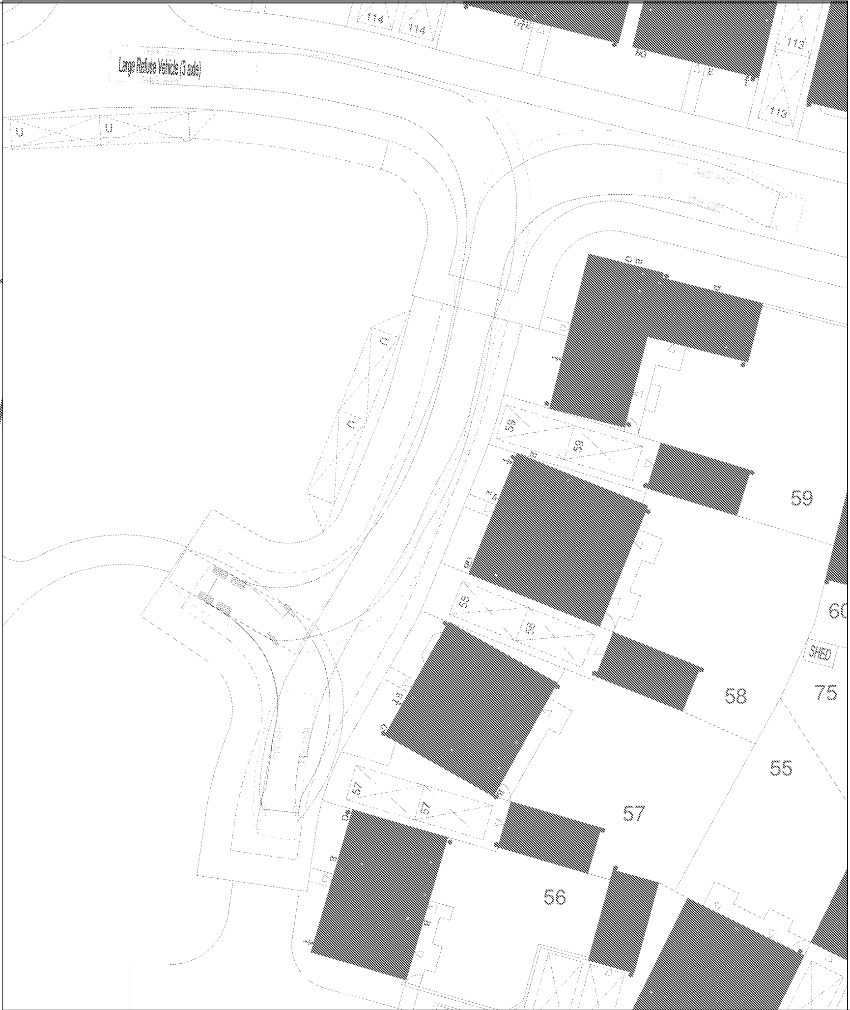
REFUSE VEHICLE TRACKING OF TURNING HEAD FOR PLOTS 52 – 59
