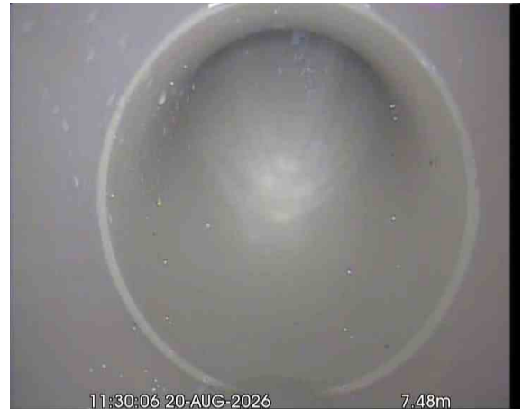
KIT. SINKX_430aaf13-ac28-47e6-9827-aef3607b2ee8_20260917_174920_910.jpg, 00:01:04, 7.48 m Line deviates up, REST BEND
