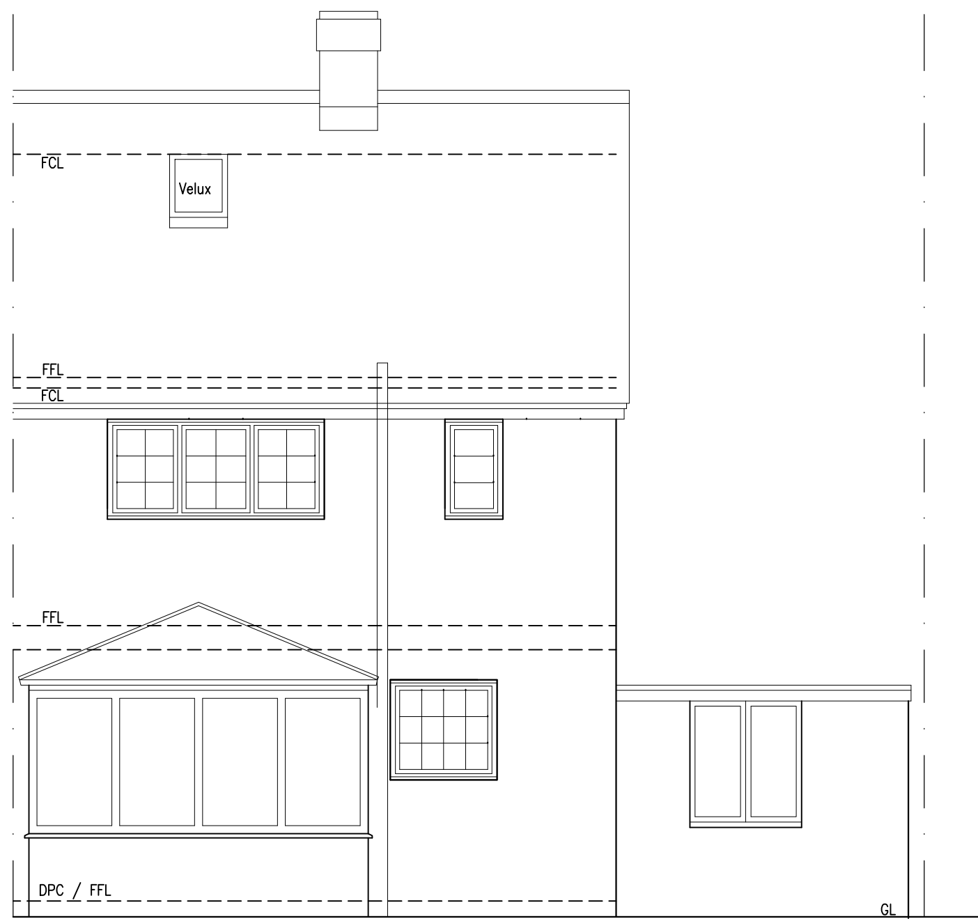
REAR ELEVATION AS EXISTING 1:50
