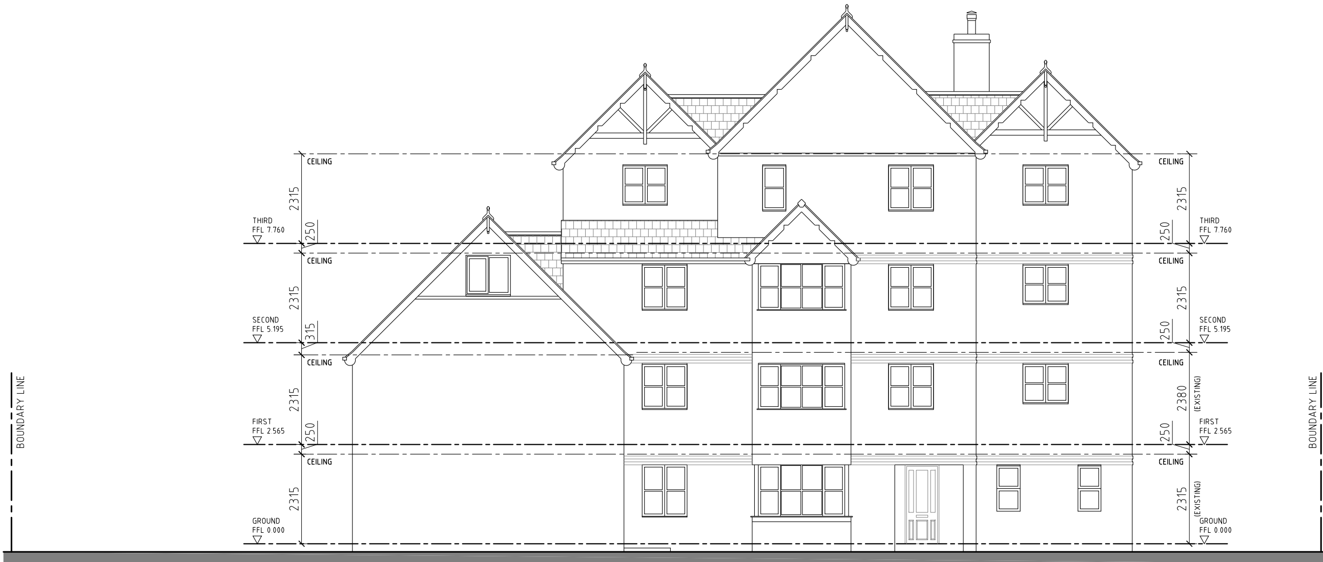
PROPOSED SOUTH-EAST ELEVATION
