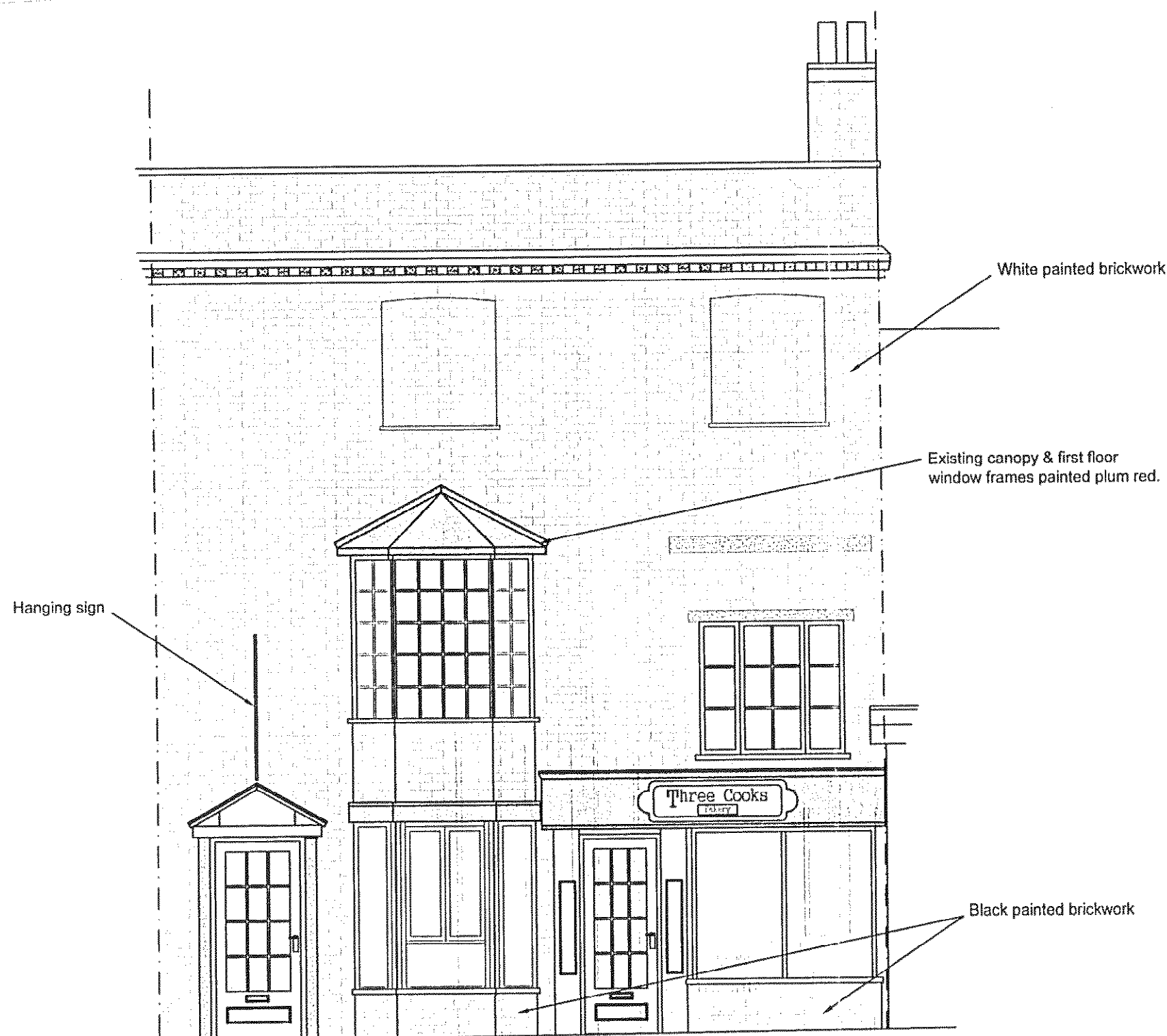
Existing Front Elevation (East). Scale 1:50
