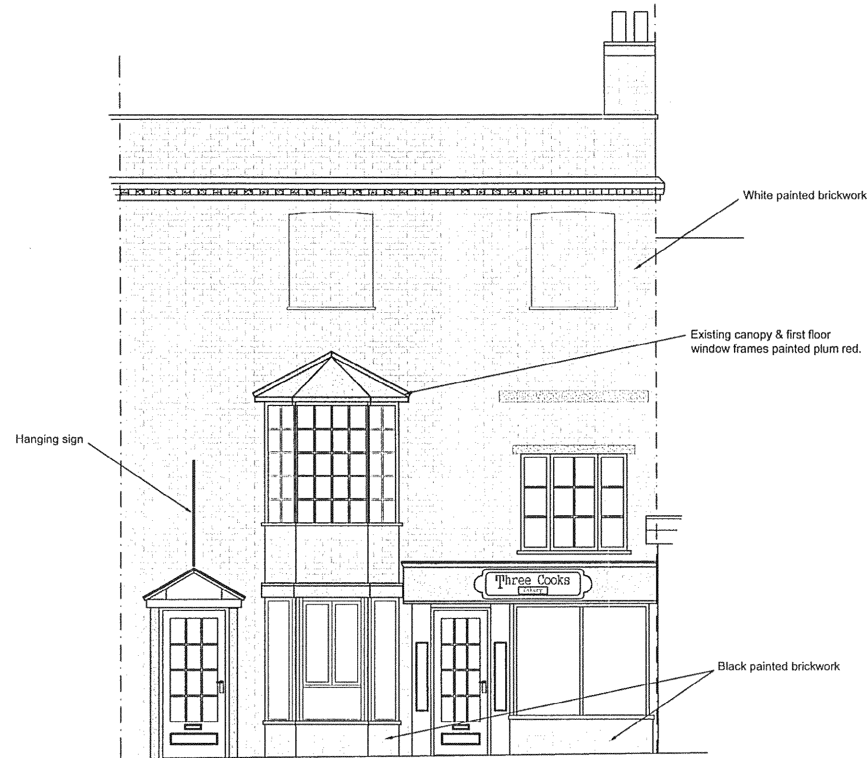
Existing Front Elevation (East). Scale 1:50
