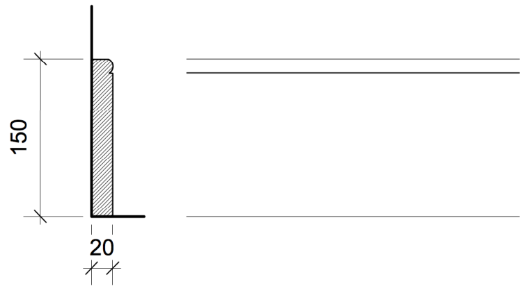
Section Elevation Routed, painted MDF Skirting: Basement and Second Floor
