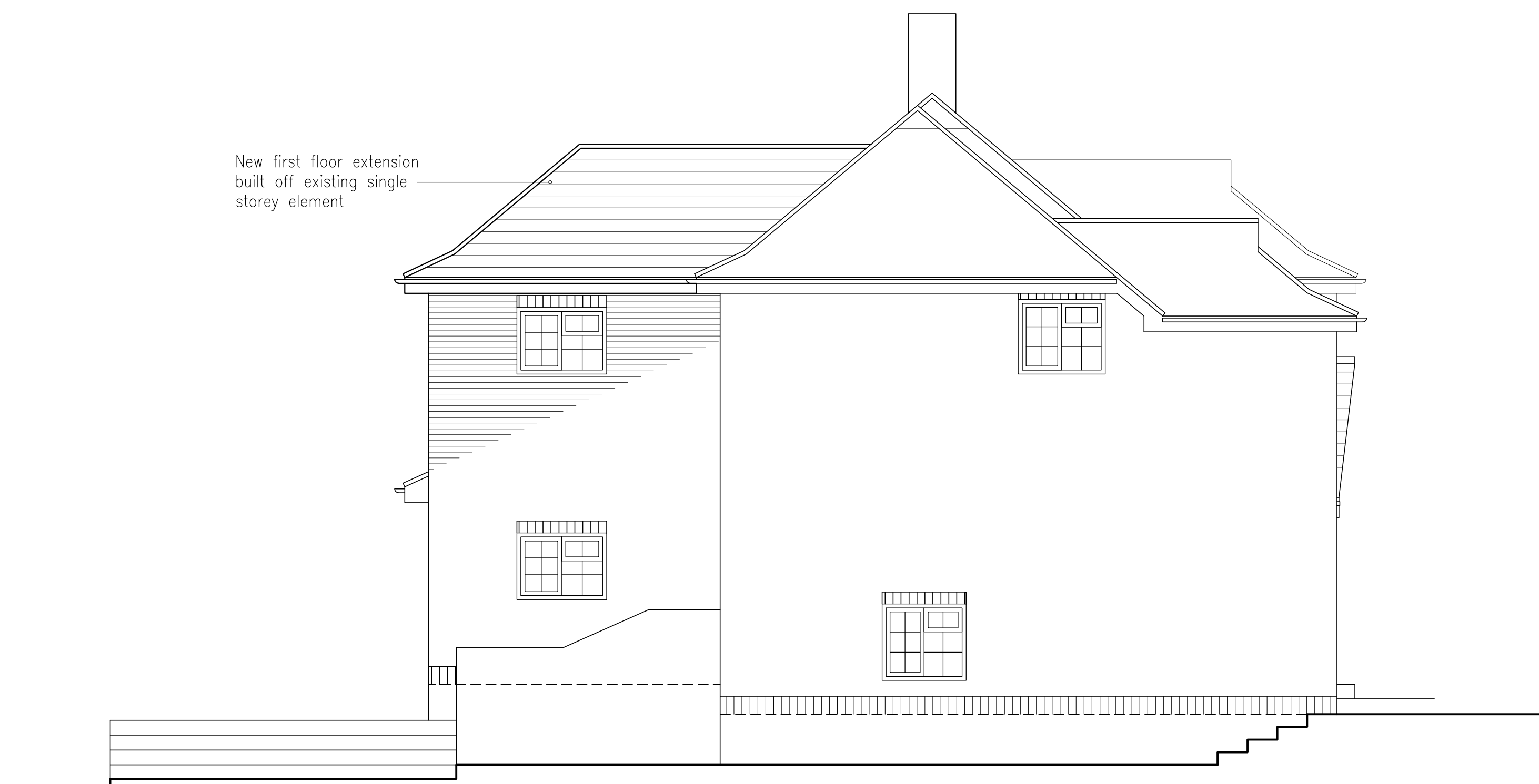
South Eastern Elevation 1:50
