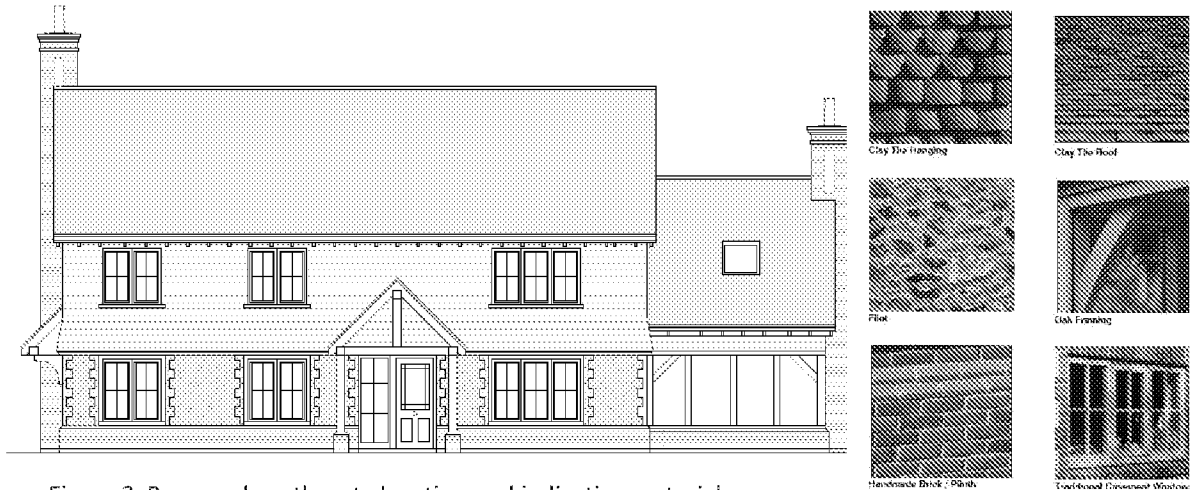
Figure 3. Proposed northeast elevation and indicative materials
