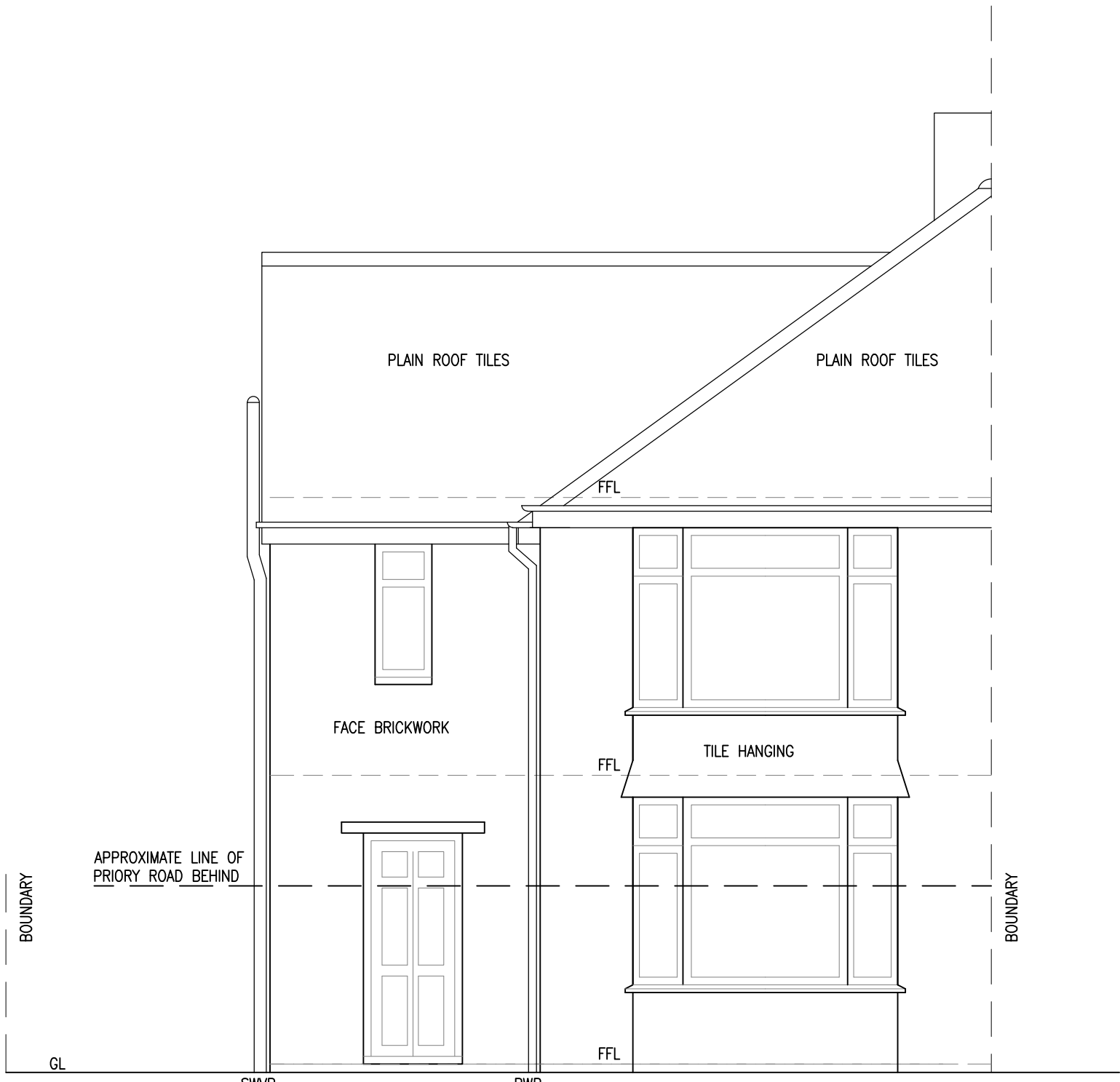
NORTH WEST ELEVATION AS EXISTING 1:50
