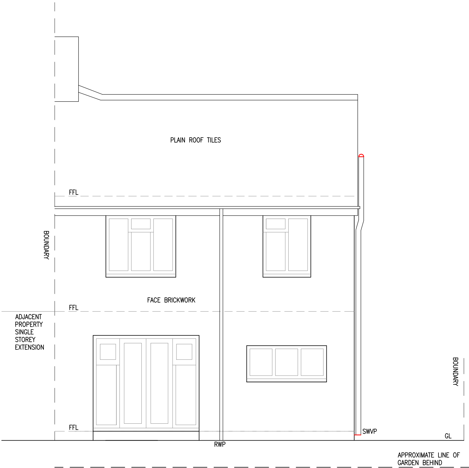
SOUTH EAST ELEVATION AS EXISTING 1:50
