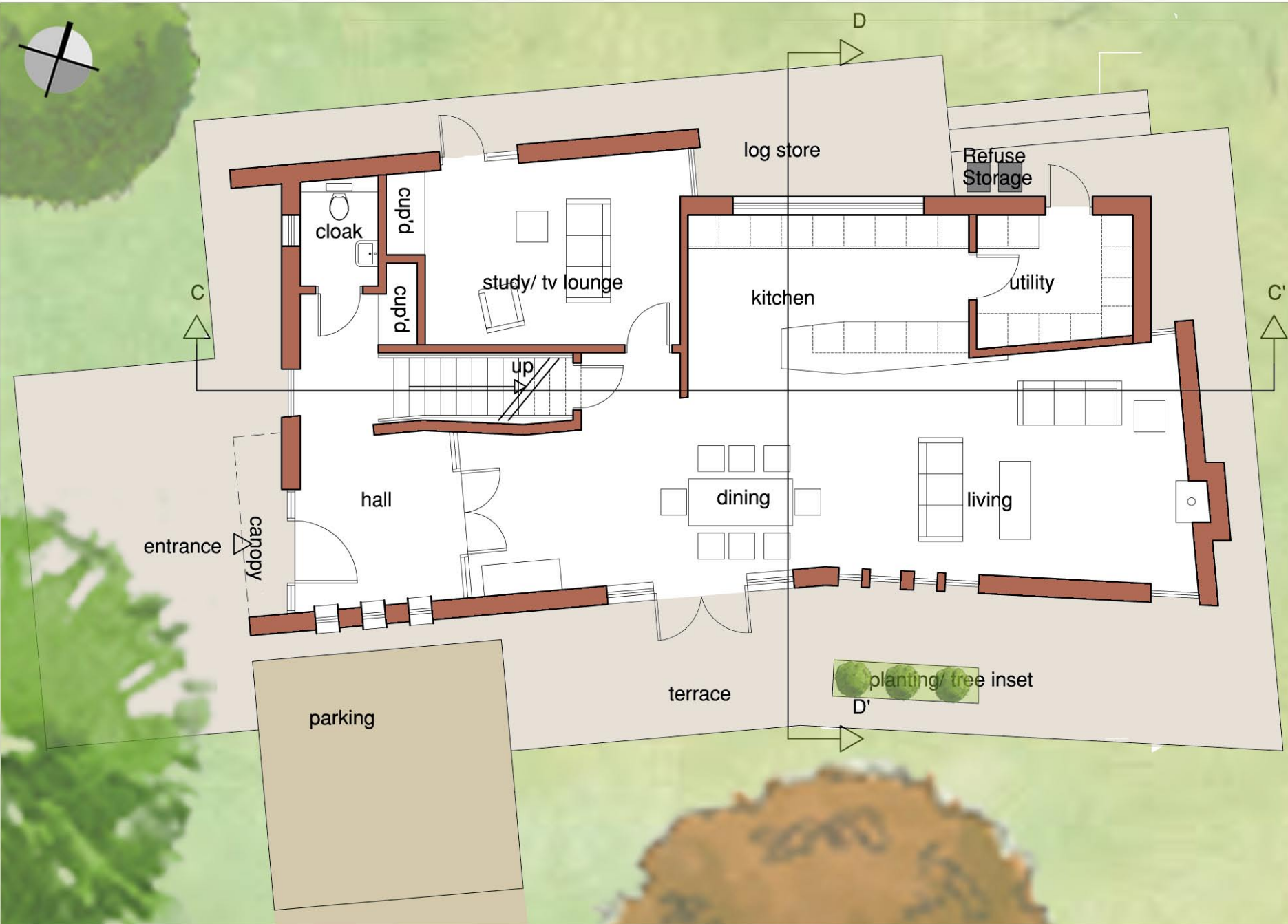
1:100 House type A- ground floor plan
