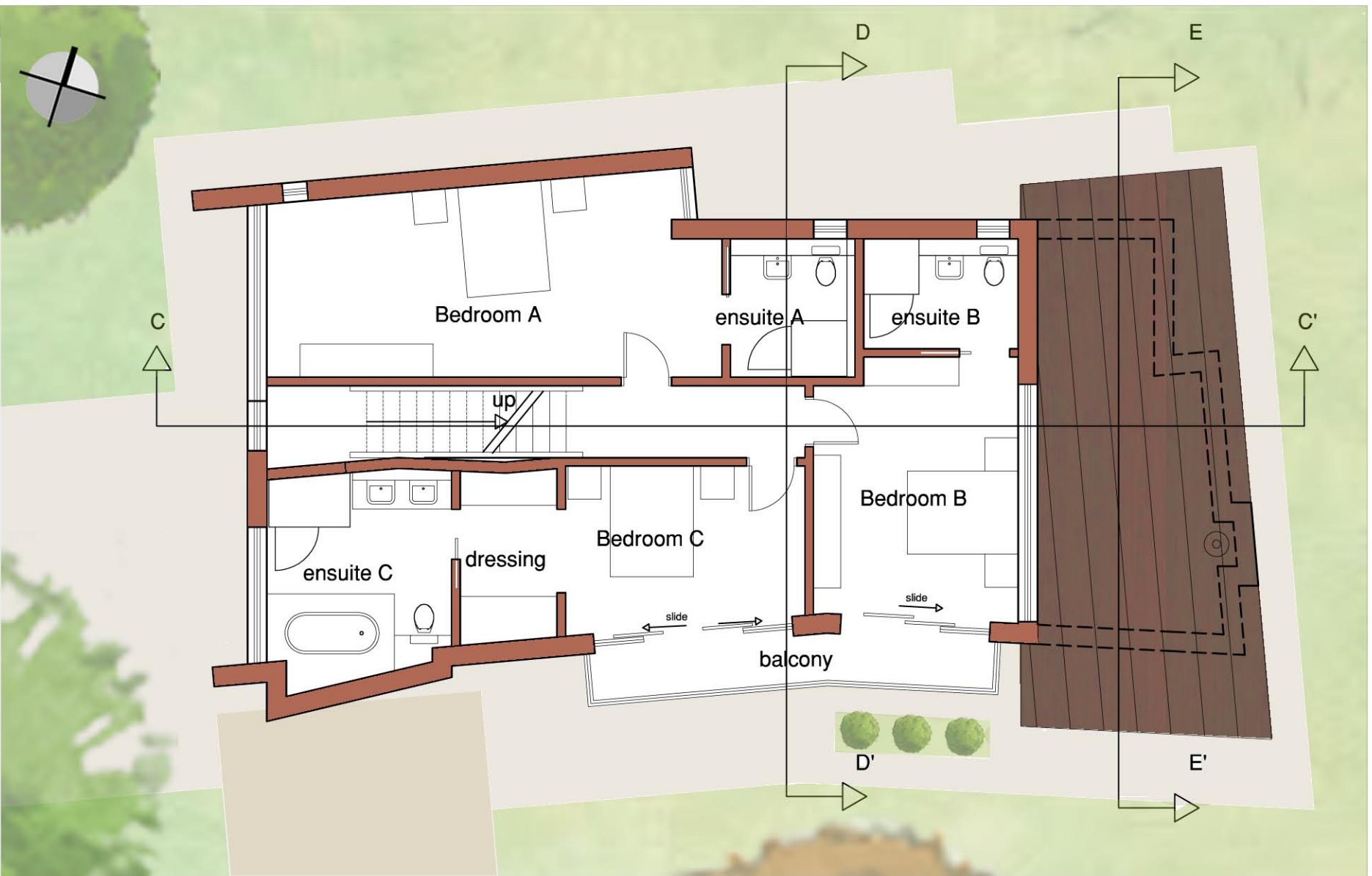
1:100 House type A - first floor plan
