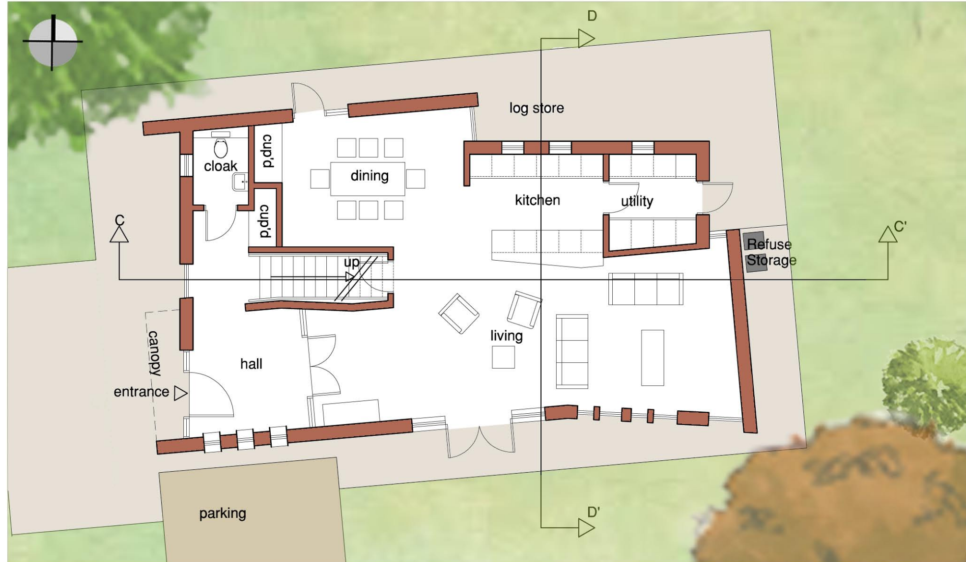
1:100 House type B (reduced size) - ground floor plan
