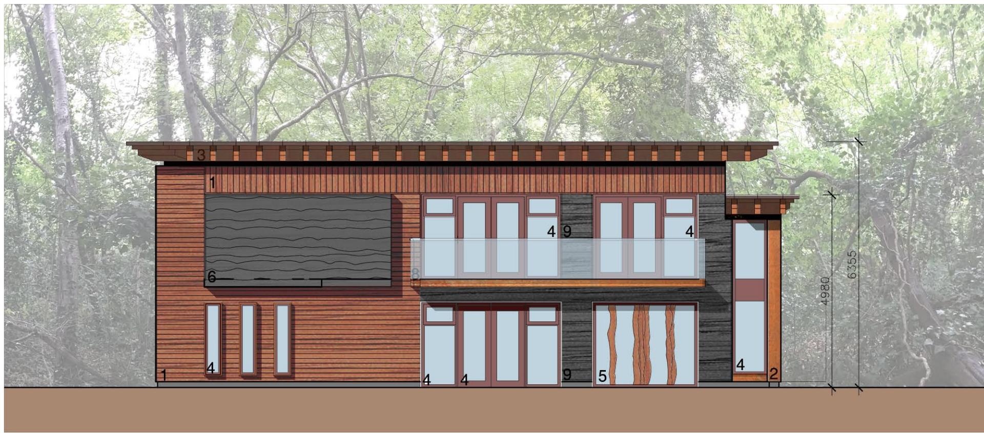
1:100 House type B- south (front) elevation
