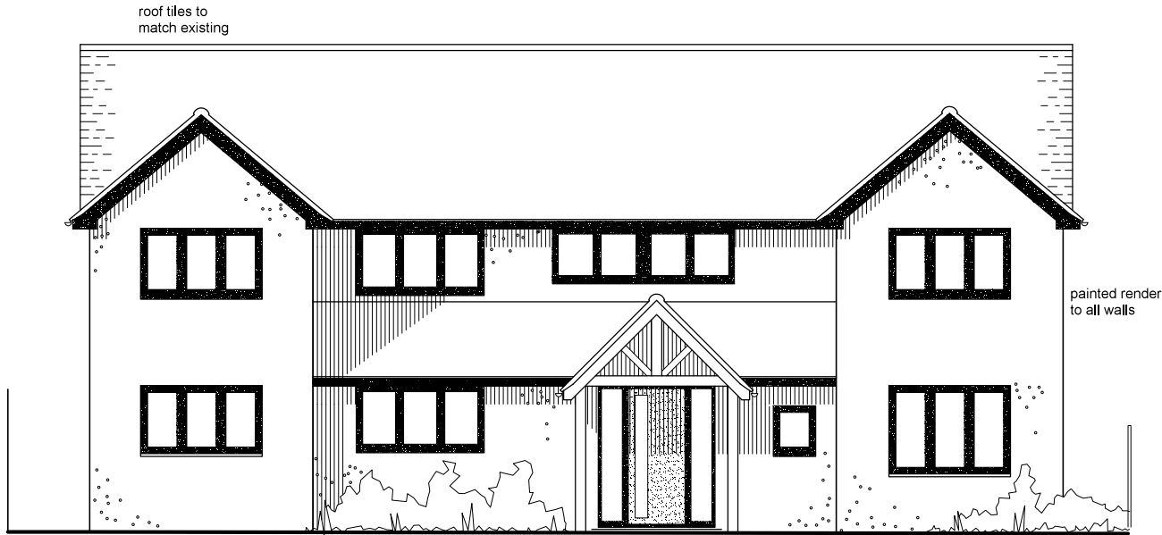
North West Elevation
