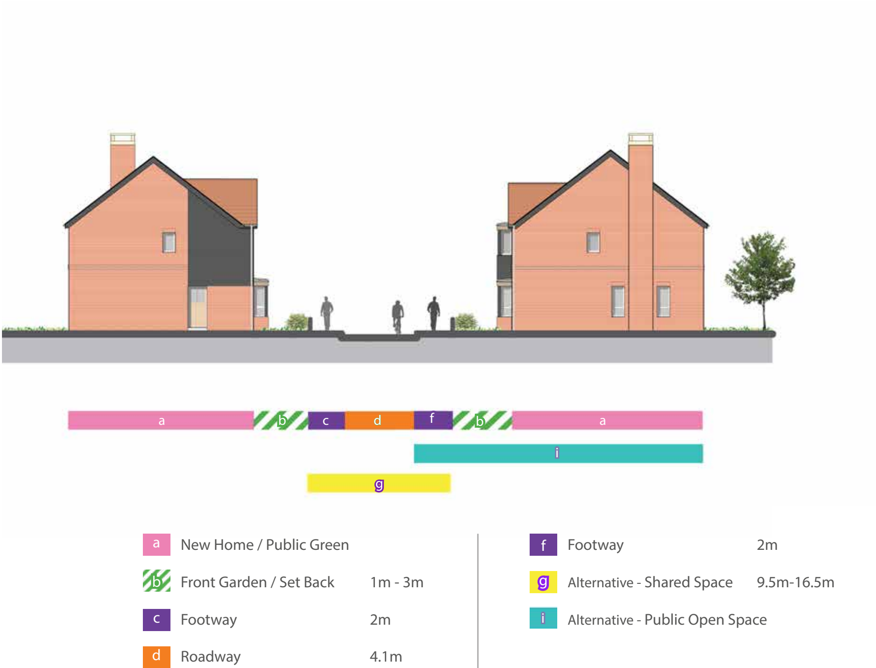
Typical shared surface lane cross section
