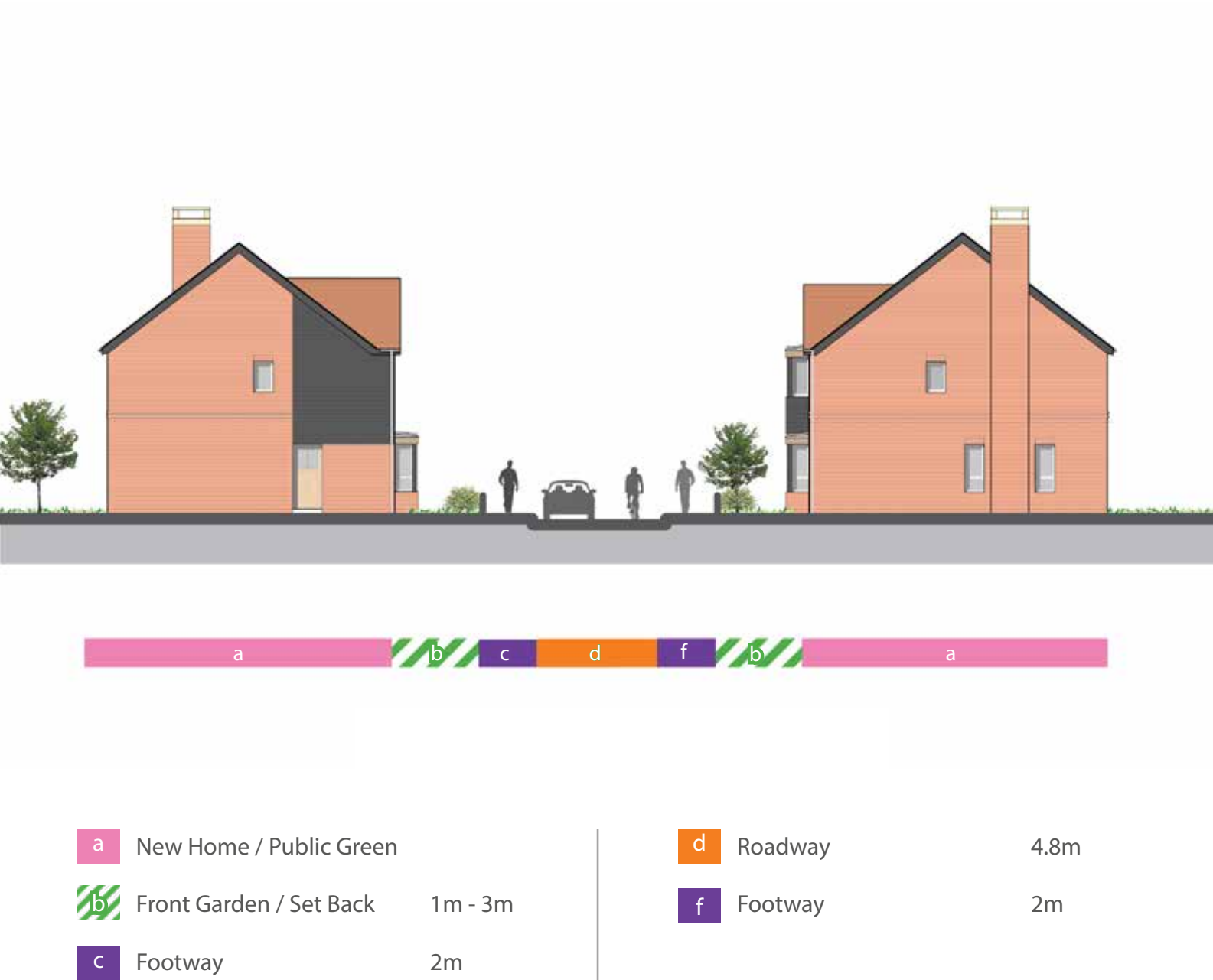
Typical secondary road cross section
