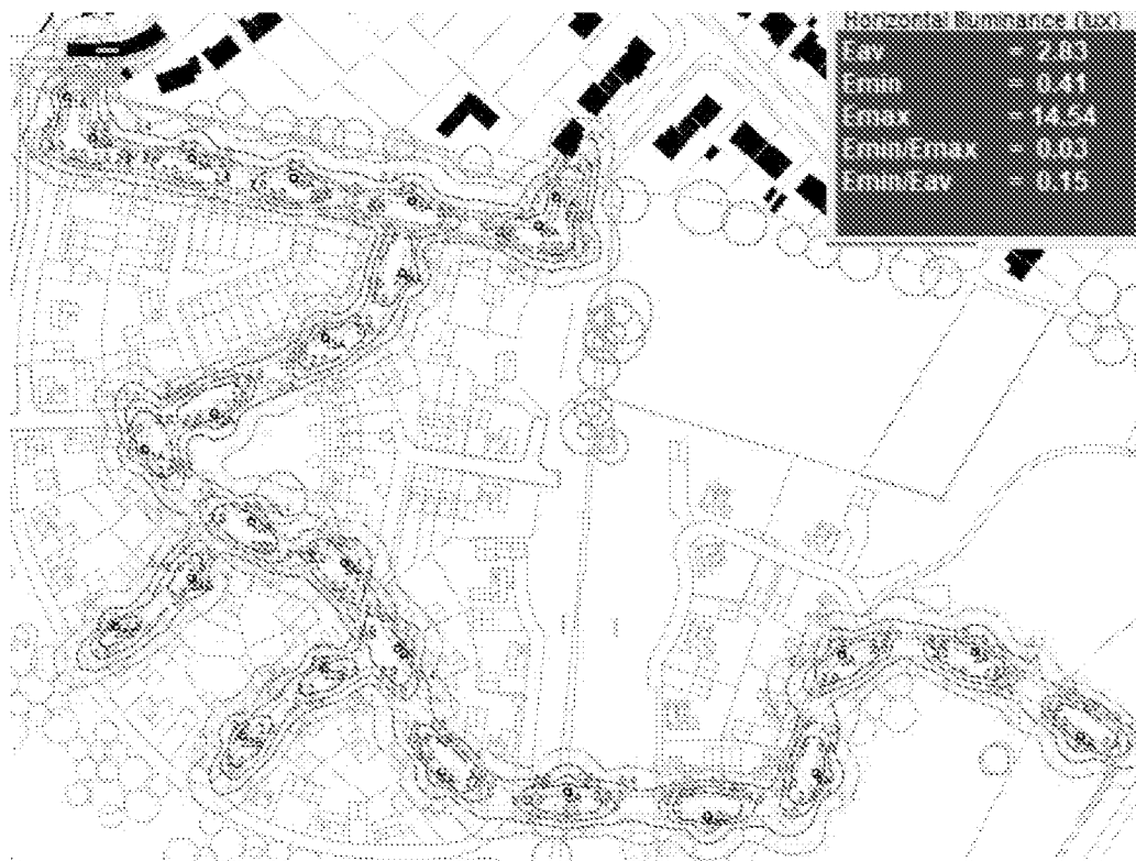
Figure 15: ISO Lux Contour Layout for Adoptable Roads
