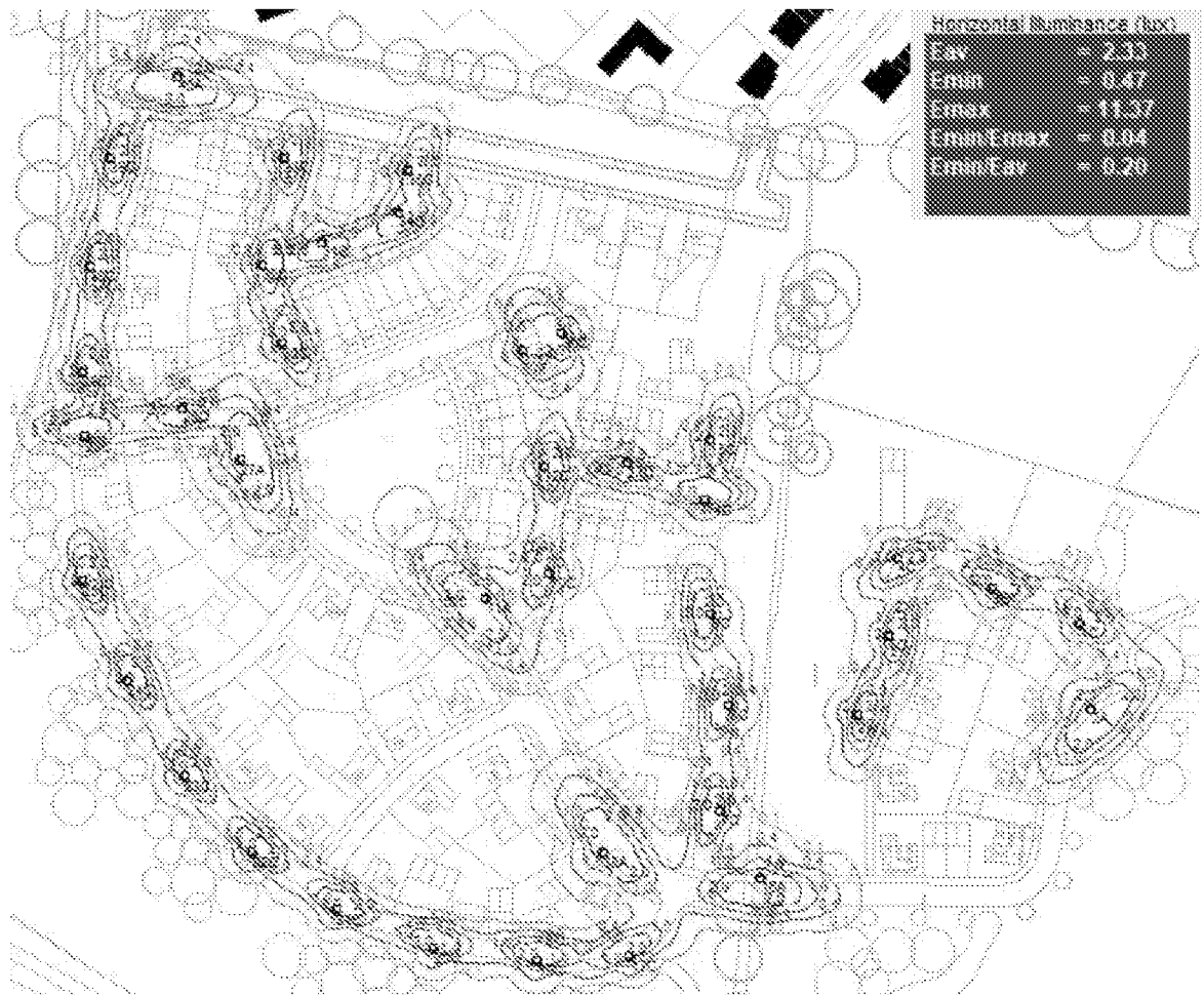
Figure 16: ISO Lux Contour Layout for Private Roads (4m Columns)
