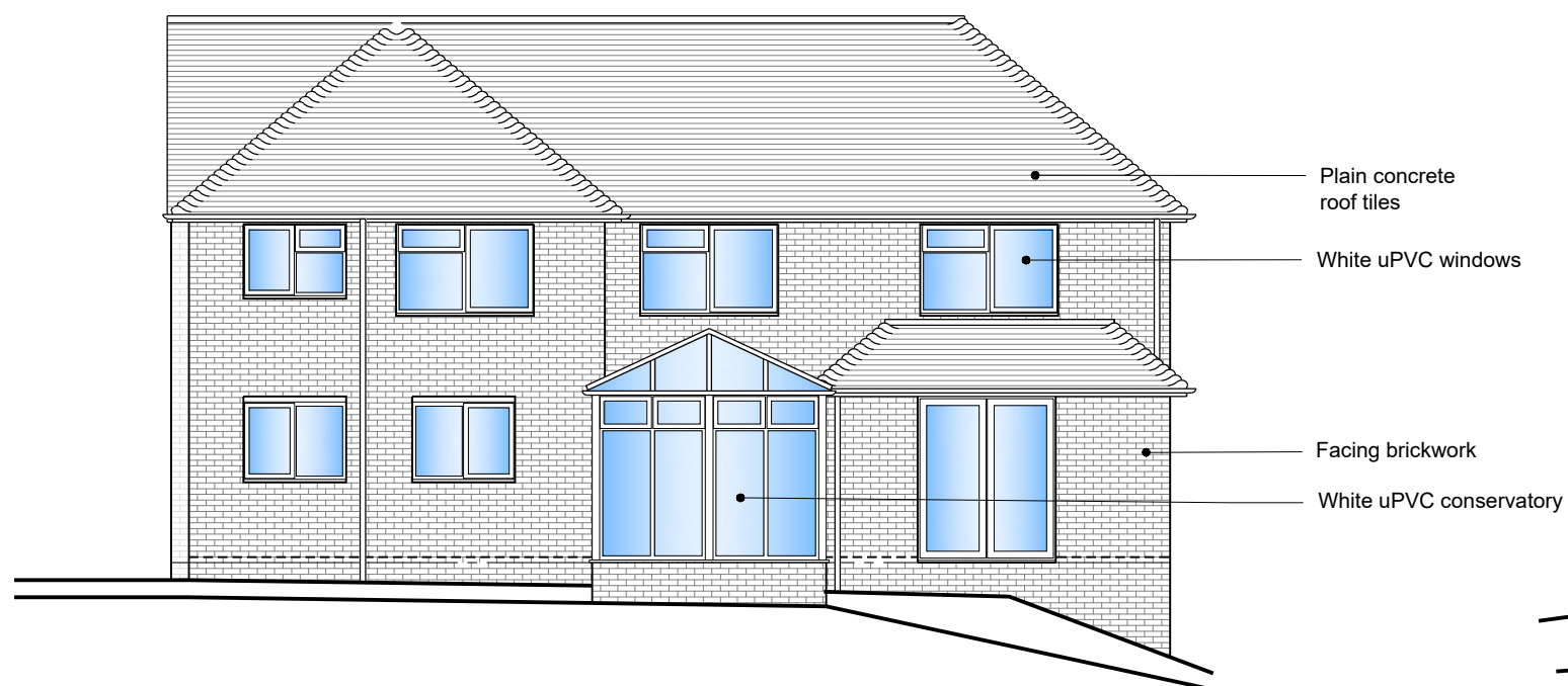
EXISTING REAR ELEVATION (SOUTH EAST)
