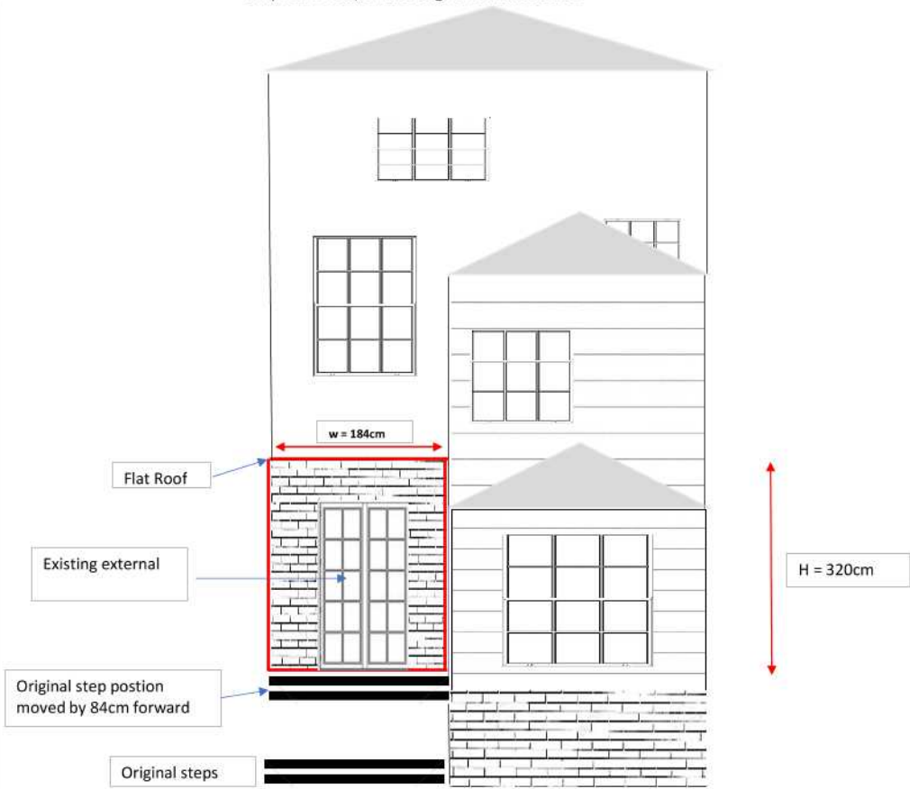
SCALE 1 to 100 Proposed Rear elevation Only red is new, all else original and untouched
