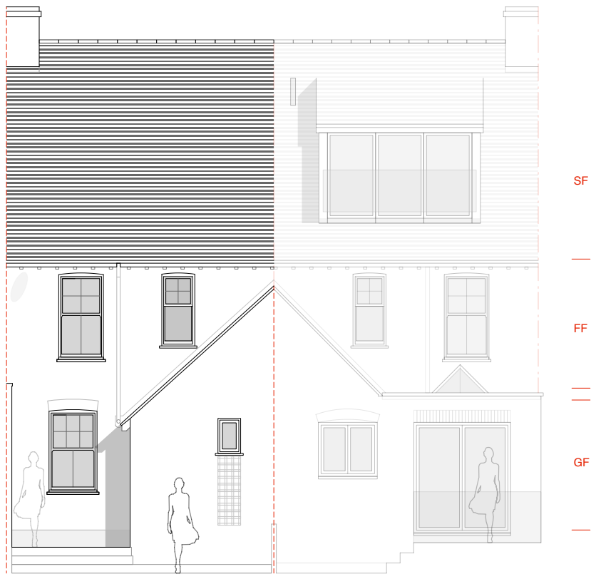
Existing Rear Elevation at 1:100 scale SOUTH EAST
